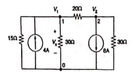
(c) Use the superposition theorem to find  $\nu$  in the circuit fig.
